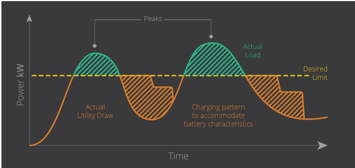
Figure 2 VPS SDP® Peak Shaving Mechanism
