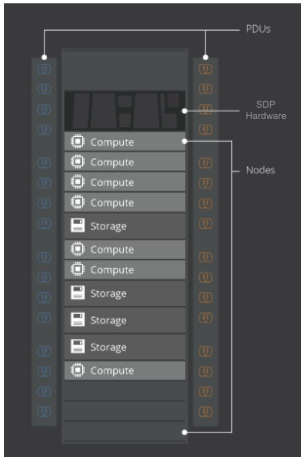
Figure 5 SDP in a Rack
