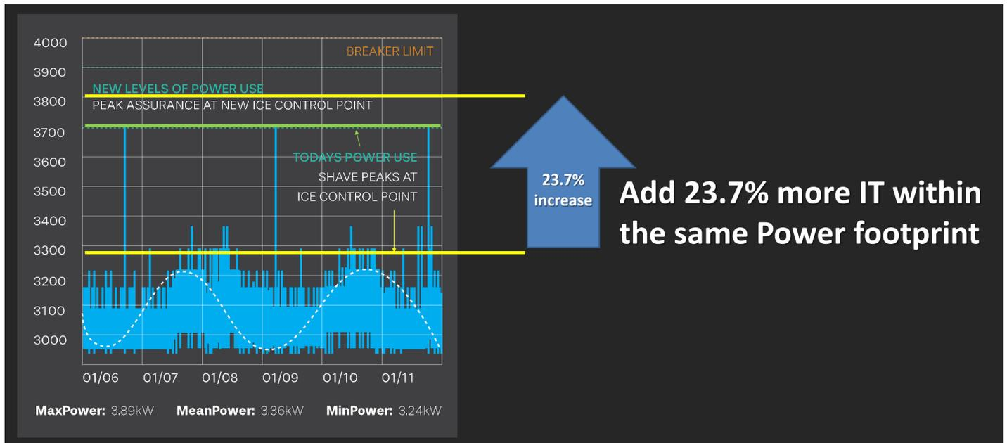
In the illustration above (taken from a large Colo provider), the average rack power (on one of the PDUs of a dual corded rack) is 3.1kW, with peaks upto 3.7kW. ICE initially caps and flattens the Grid power draw to a control limit of 3.3 kW. This allows deployment of more IT servers in the rack and increased baseload of 23.7%. The same concept is extrapolated to a Row or entire Data Center.
