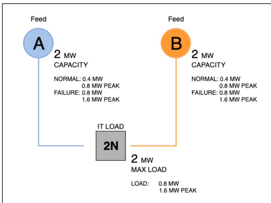
Figure 3: Redundant power paths to 2N workloads in a data center.
