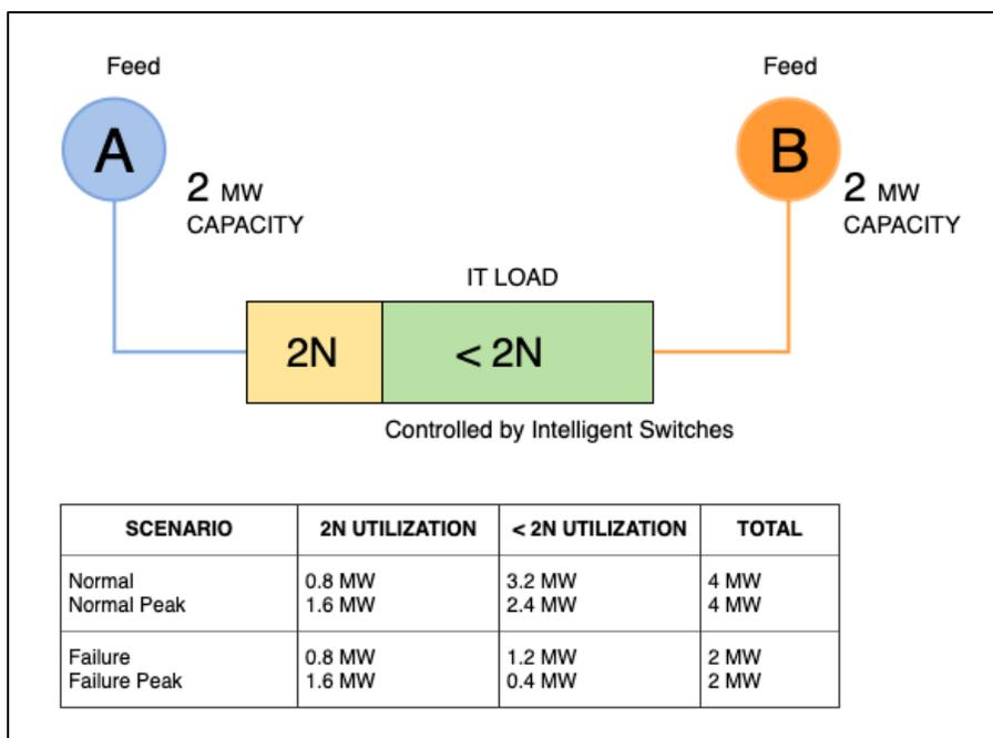
*Figure 4: Capacity unlocked by dynamic redundancy*
