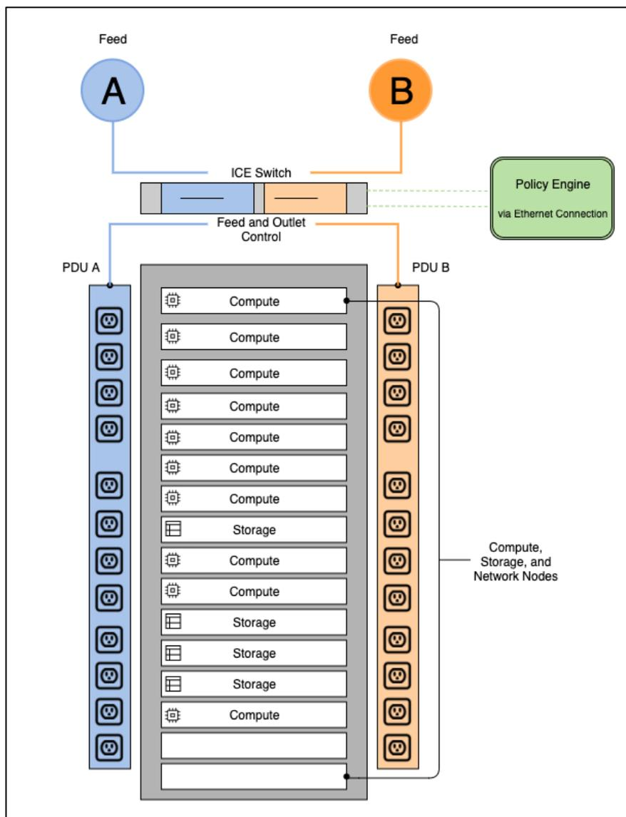
Figure 2: Power switch at the top of a rack controlling redundant power feeds
